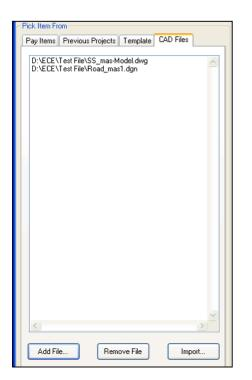
Click the *Add File...* button and select the CAD files (\*.DWG, \*.DXF and \*.DGN) that contain the pay items for the cost estimation. All existing files are provided in the list box.
